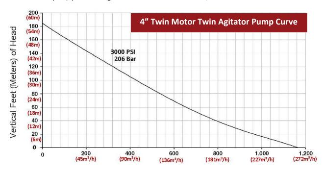
GPM (m³/h) Pumping Water
