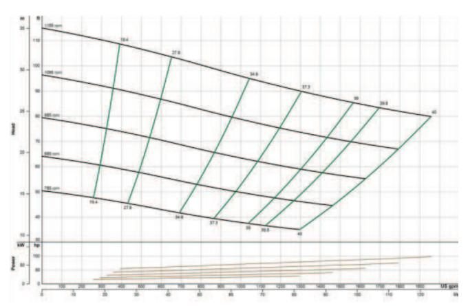
\*General pump curve based on water at 1200 RPM. Contact us with your specific material for a custom pump curweve.
