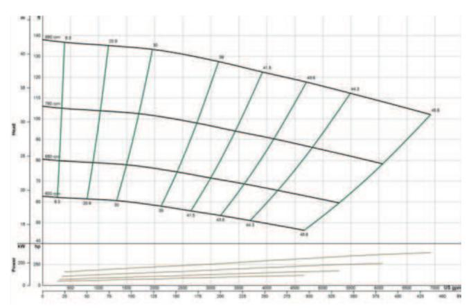
\*General pump curve based on water with 1200 RPM motor. Contact us with your specific material for a custom pump curve.
