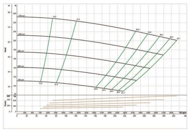
\*General pump curve based on water with 1200 RPM motor. Contact us with your specific material for a custom pump curve.
